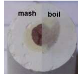
Figure 15 - For experiment 28 (mash pH 4.55) the wort at the end of the mash and the beginning of the boil was tested for starch and both tested positive
