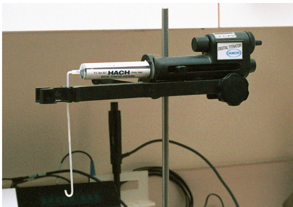
Figure 2.2 Digital Titrator. Shown here mounted to stand via mounting fixture which can also accomodate pH electrode, RTD. Can also be operated hand held in which case a straight dip tube is used
