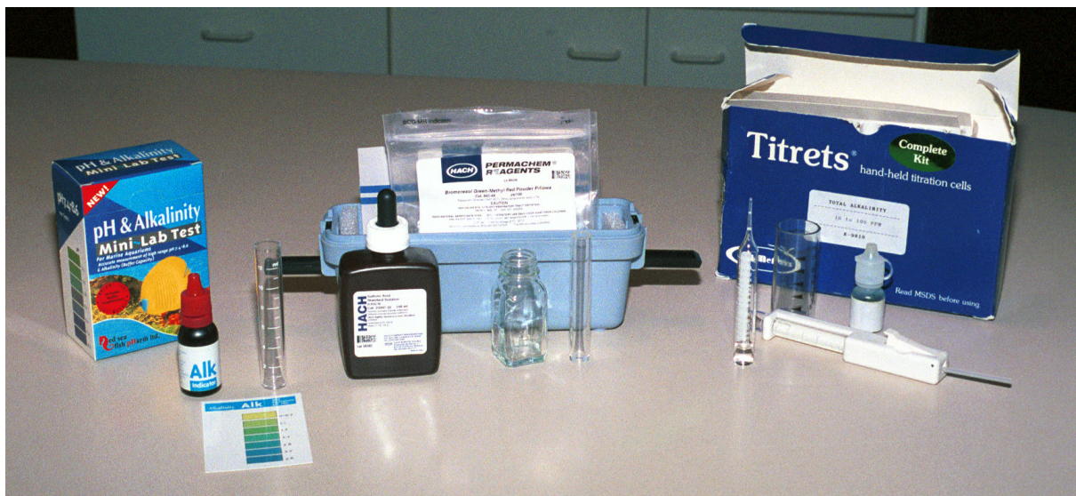
Figure 2.3 Alkalinity Test Kits. Left to right: Aquarium, Drop Titration, Reverse Titration Evacuated Ampoule
